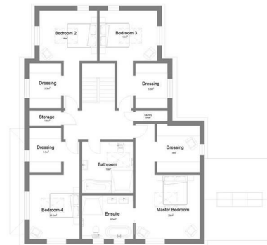
Proposed First Floor Plan Scale @ 1:100
